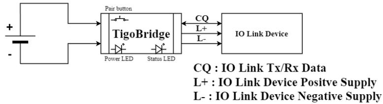
Figure 6 - Electrical Schematic Diagram
