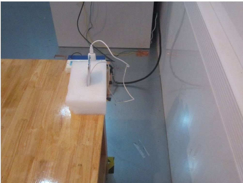
Conducted Emissions Test Setup Side View
