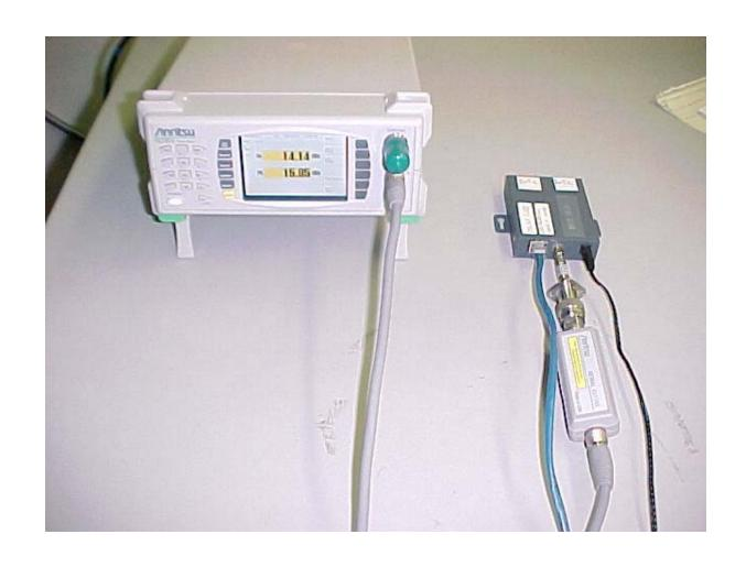
Maximum Peak Output Power Measurement Setup
