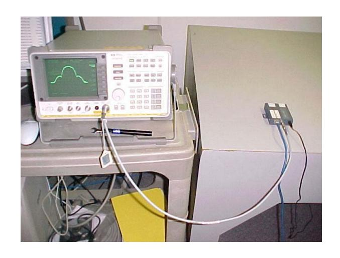
Conducted Emissions at Antenna Terminal Setup
