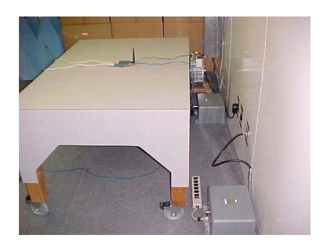
AC Conducted Emissions Measurement (Rear View) Setup
