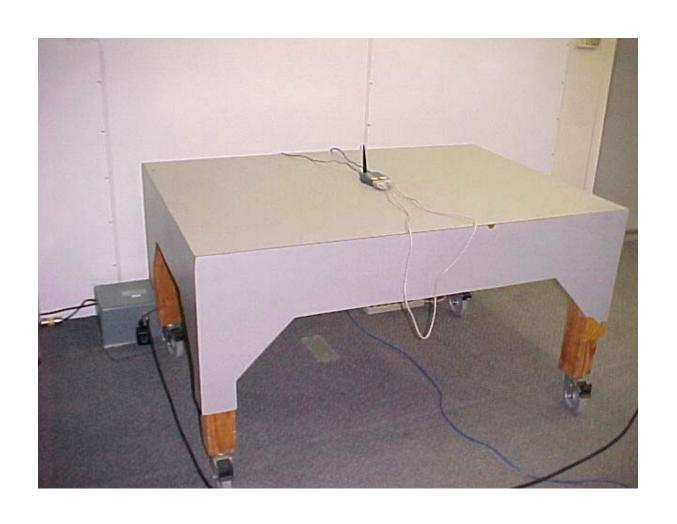
AC Conducted Emissions Measurement (Front View) Setup
