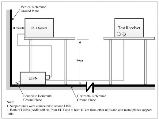
The measurement was performed at shield room, using the setup per ANSI C63.10-2013 measurement procedure. The specification used were FCC §15.207 limits.
