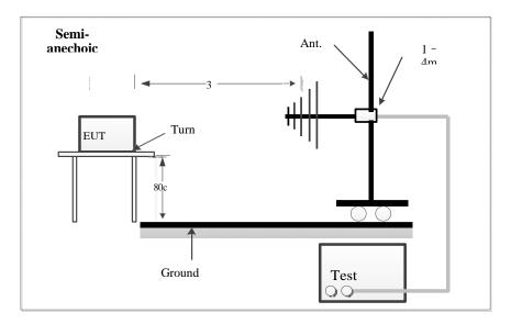
The radiated emissions tests were performed in the 5-meter Chamber, using the setup in accordance with ANSI C63.10-2013. The specification used was the FCC 15 Subpart C limits.
