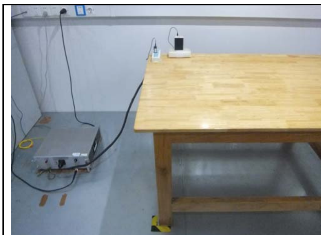
Conducted Emissions Test Setup Front View
