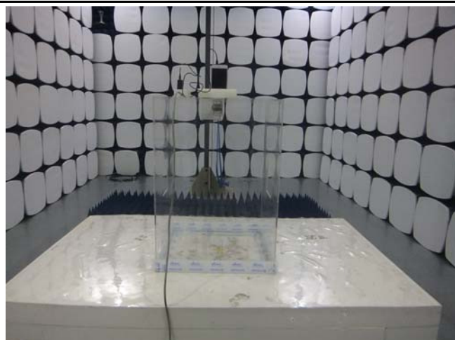
Radiated Spurious Emissions Test Setup Above 1GHz
