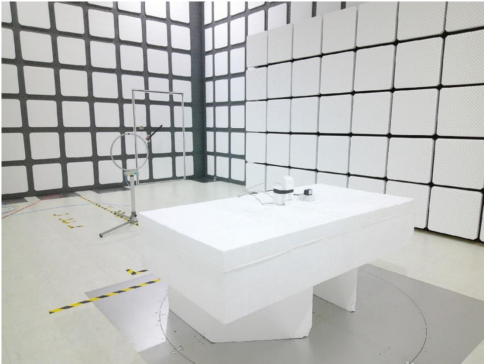
Description: Radiated Emission Test Setup for 30MHz~1GHz
