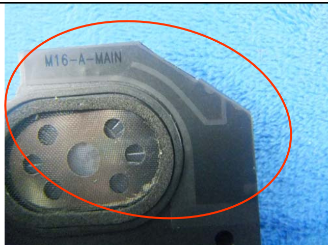
GSM/PCS/UMTS-FDD Antenna View
