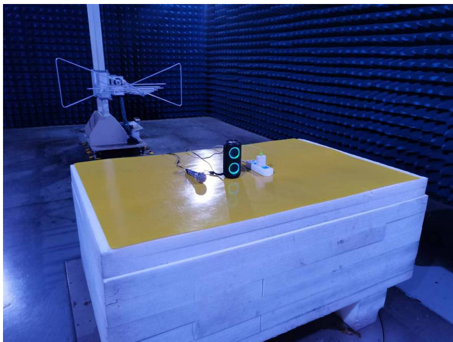
Photo of Radiated Emission Measurement (Above 1G)
