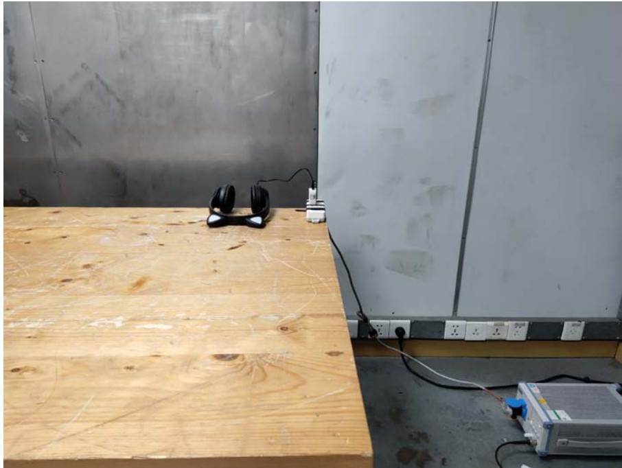
Photo of Power Line Conducted Emission Measurement
