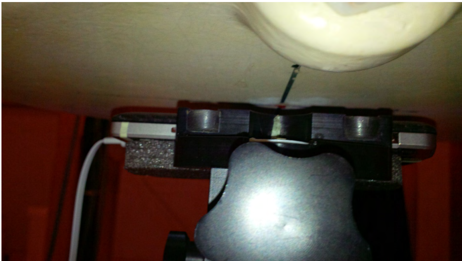
Figure E10. Body-worn configuration (No Holster, headset, back 10mm away)
