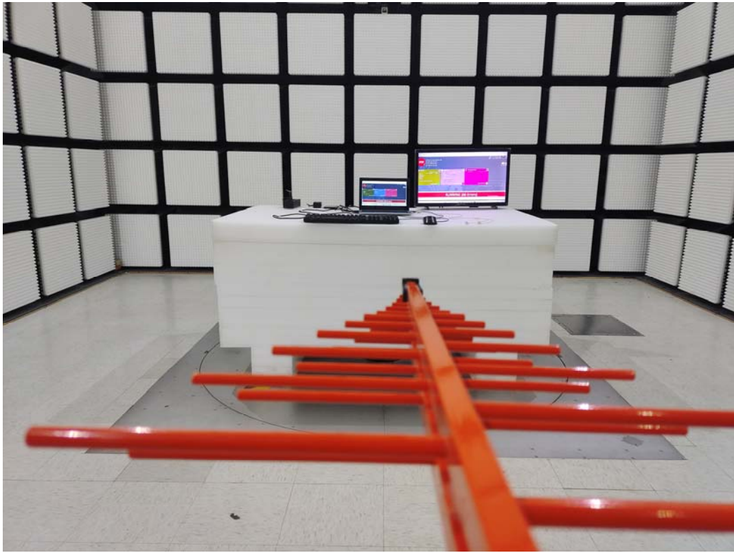
Radiated Emission Above 1GHz View
