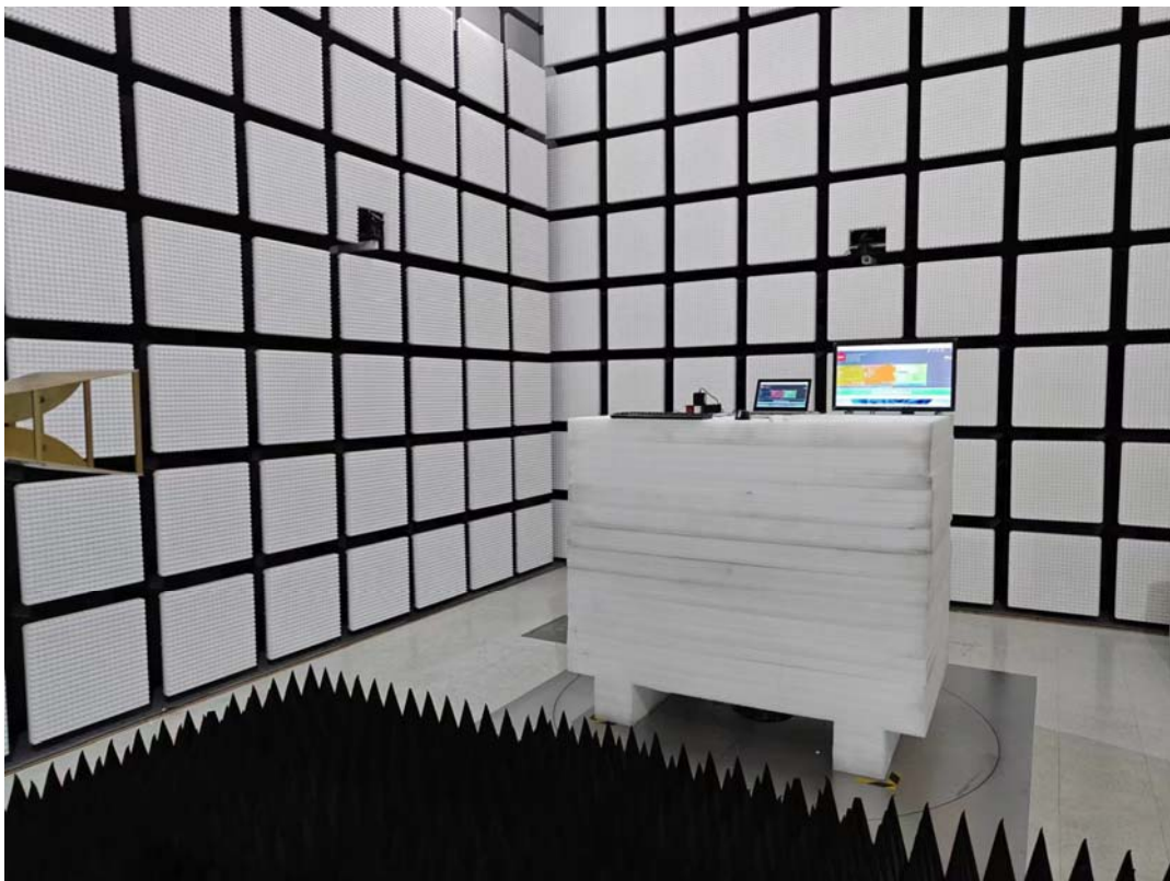
Radiated Emission Above 1GHz View
