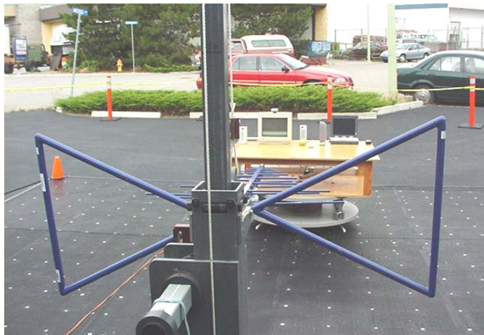
Photograph F-3 - Front of Radiated Emission Configuration
