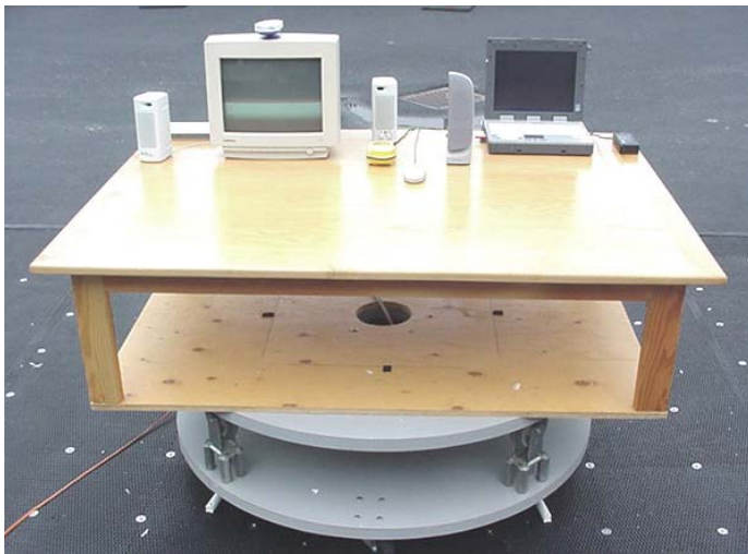
Photograph E-3 - Front of Radiated Emission Configuration
