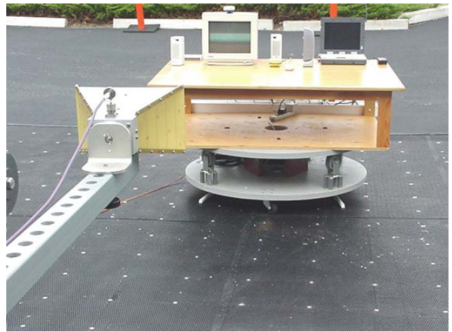
Photograph F-4 - Back of Radiated Emission Configuration
