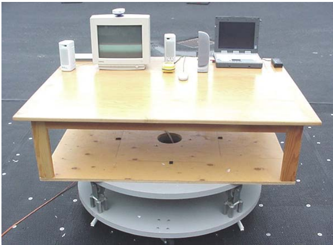
Photograph F-3 - Front of Radiated Emission Configuration
