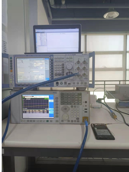
'RF Conducted Test setup (GSM/WCDMA/LTE)
