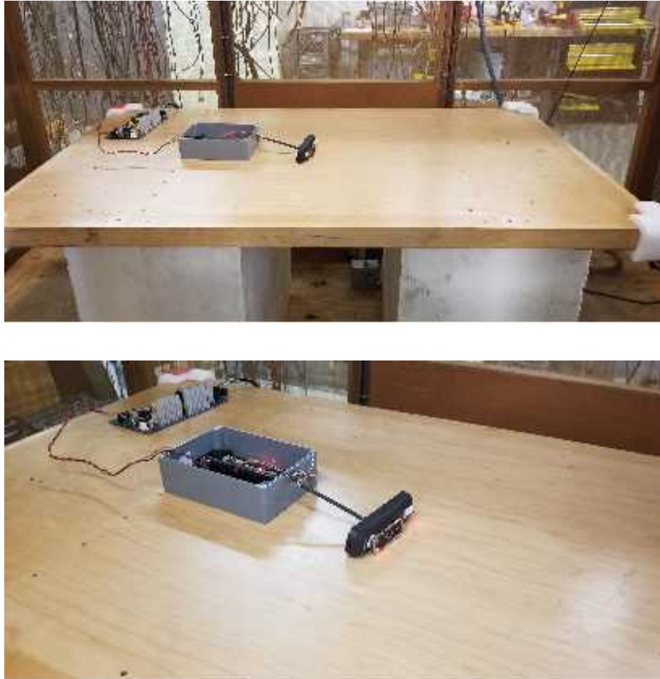
Figure 6: Conducted Emissions Test Setup Photograph(s).
