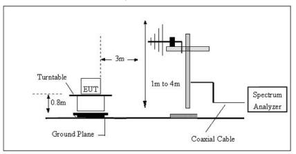
(C) Radiated Emission Test-Up Frequency Above 1GHz
