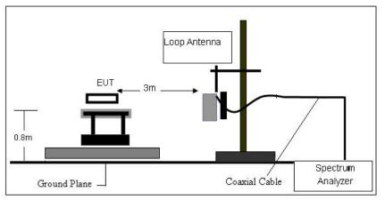
(B) Radiated Emission Test-Up Frequency 30MHz~1GHz
