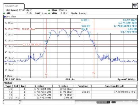
26dB Bandwidth and 99% Occupied Bandwidth Plot on Configuration IEEE 802.11n MCS0 HT20 / Chain 1 + Chain 2 / 5785 MHz
