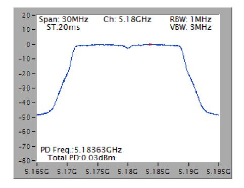
Power Density Plot on Configuration IEEE 802.11a / Chain 1 / 5180 MHz
