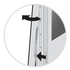
2. Press and hold the rotate buttons while moving the arms back towards the wall
