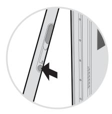
3. Press the rotate button along each arm
