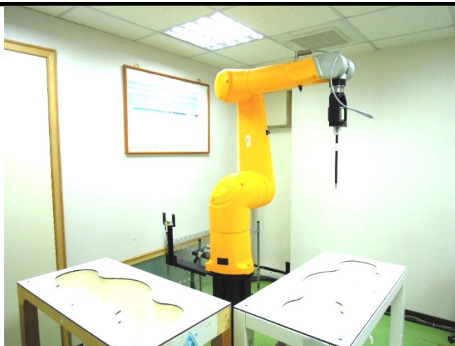
Fig-3.2 SPEAG DASY52 System
