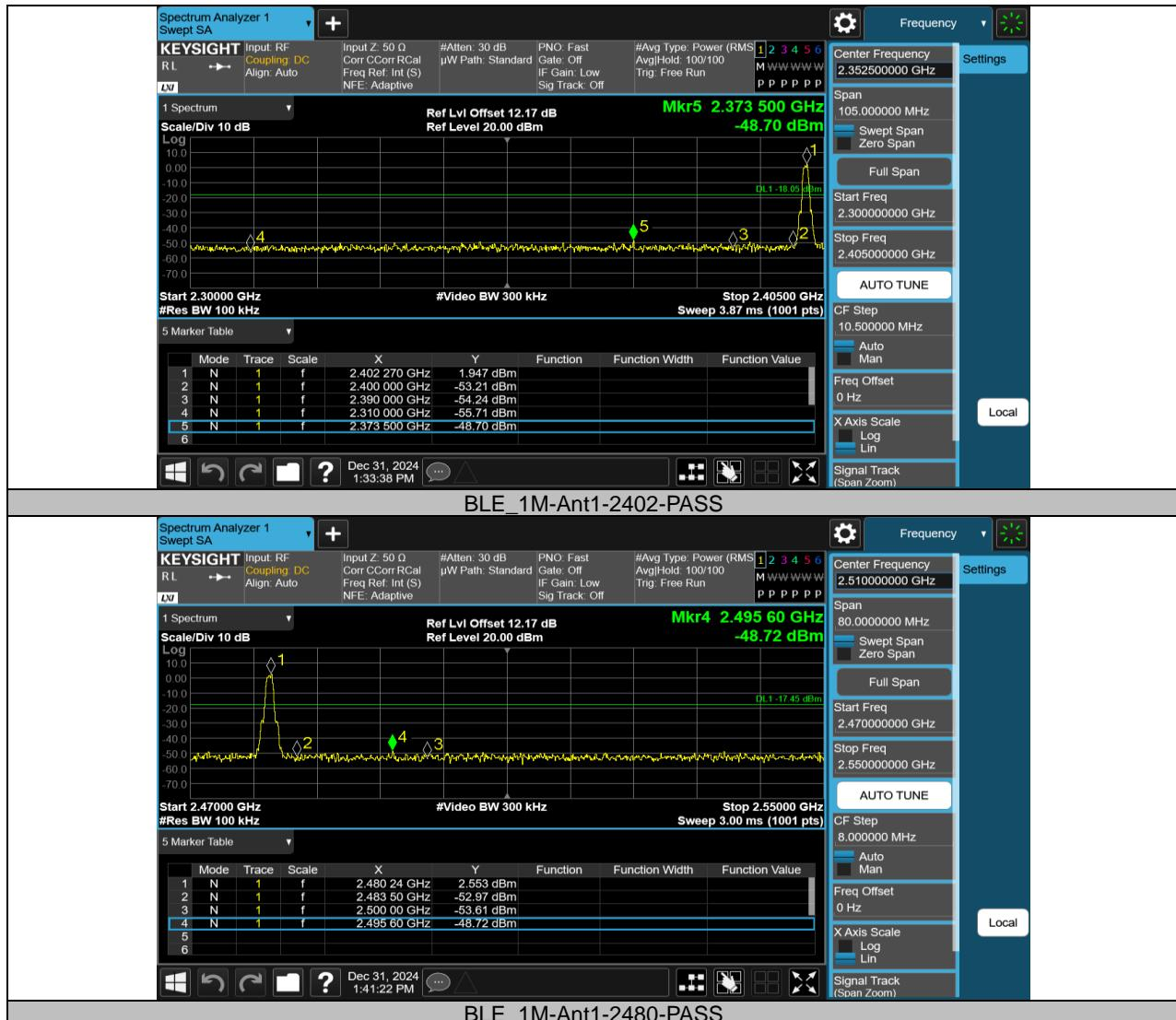
**TEST REPORT****Conducted Spurious Emission****Test Result**
