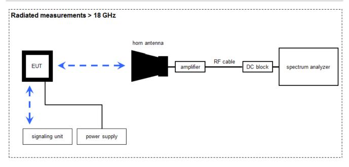
Measurement distance: horn antenna 50 cm
