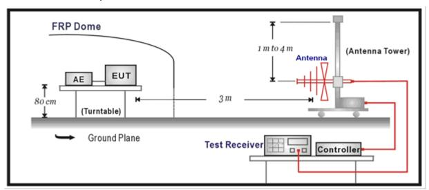
Above 1GHz Test Setup:
