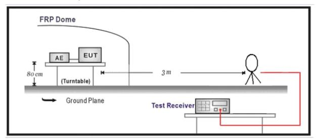
Below 1GHz Test Setup:
