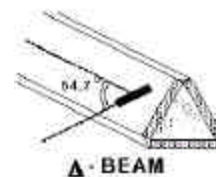
Figure 3.1 Triangular Probe Configuration
