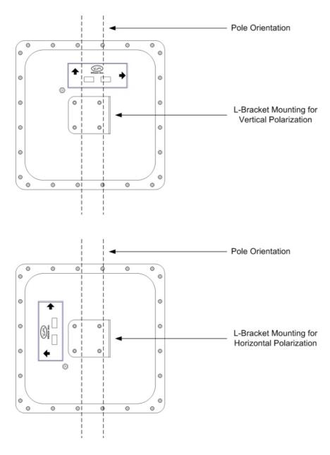
Once the L-bracket is in place, the unit can be mounted to the pole. The pole catch, V-bolt and L-bracket are oriented as shown in Diagram 2.2B.
