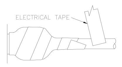
When done, the connection should be tightly wrapped with tape, with a good seal to the cable.
