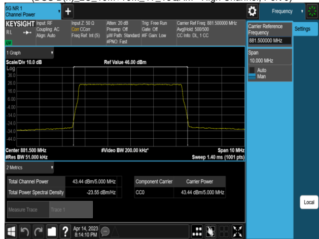
Plot 8-144. Conducted Average Output Power Plot (NR n5_1C_5M_4T_256QAM - Middle Channel, Port 0)
