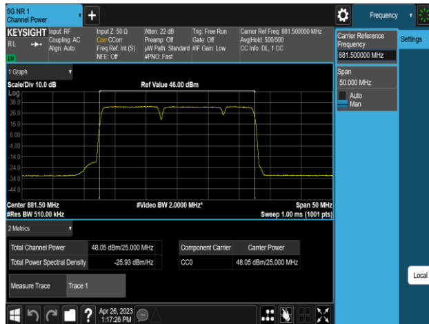
Plot 8-129. Conducted Average Output Power Plot (MSR 3C_DSS B(n)5_1C_10M+NR n5_1C_10M+LTE B5_1C_5M_2T_QPSK - Middle Channel, Port 1)
