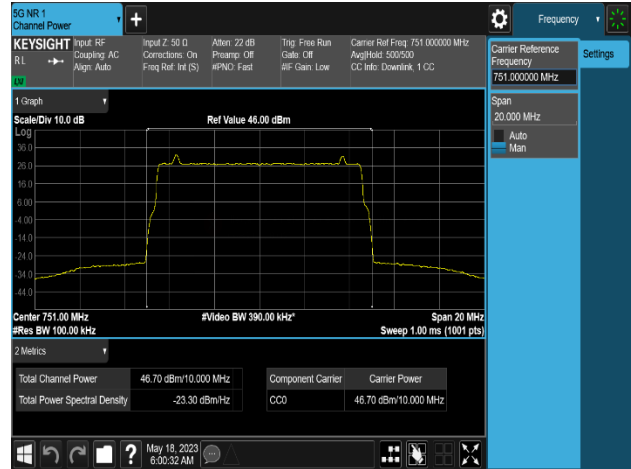
Plot 8-184. Conducted Average Output Power Plot (LTE_B13_10M(LTE)+NB-IoT(2IB)_1C_4T_QPSK - Mid Channel, Port 3)
