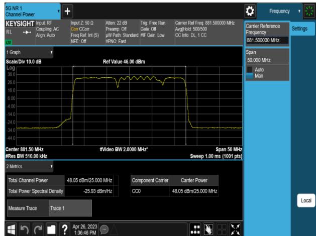
Plot 8-130. Conducted Average Output Power Plot (MSR 3C_DSS B(n)5_1C_10M+NR n5_1C_10M+LTE B5_1C_5M_2T_16QAM - Middle Channel, Port 1)
