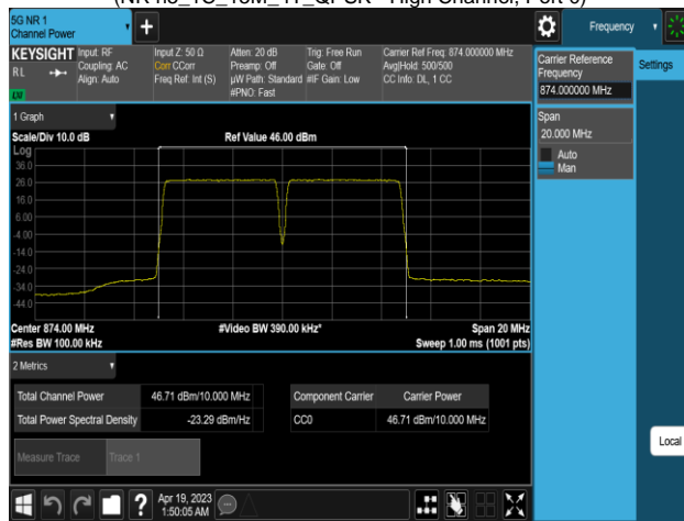
Plot 8-149. Conducted Average Output Power Plot (NR n5_2C_5M+5M_4T_QPSK - Low Channel, Port 0)
