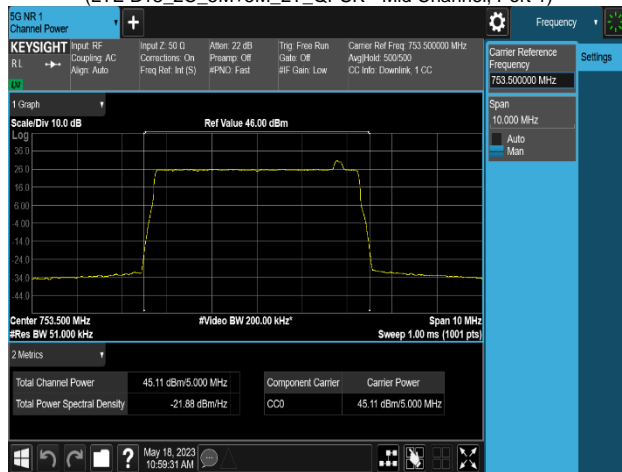
Plot 8-175. Conducted Average Output Power Plot (LTE_B13_5M(LTE)+NB-IoT(11B)_1C_2T_QPSK - Mid Channel, Port 1)
