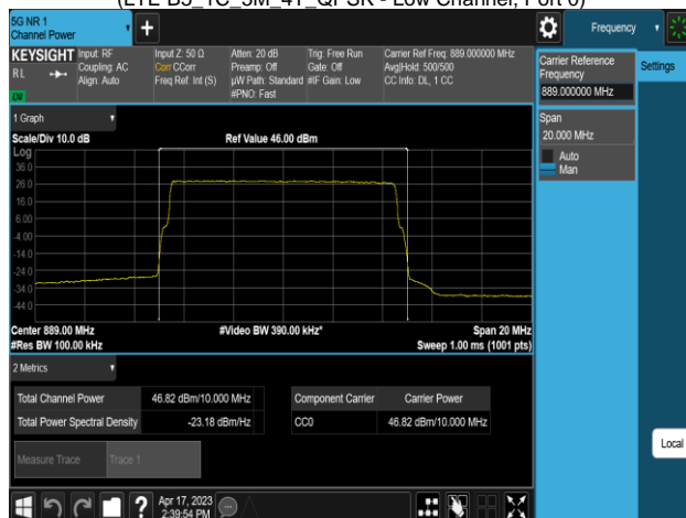
Plot 8-133. Conducted Average Output Power Plot (LTE B5_1C_10M_4T_QPSK - High Channel, Port 0)
