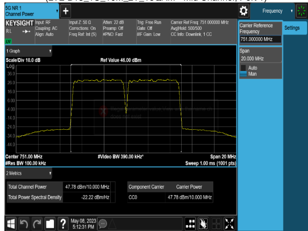
Plot 8-174. Conducted Average Output Power Plot (LTE B13_2C_5M+5M_2T_16QAM - Mid Channel, Port 1)
