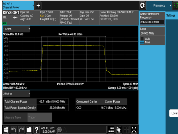
Plot 8-147. Conducted Average Output Power Plot (NR n5_1C_15M_4T_QPSK - High Channel, Port 0)
