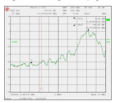
Zigbee Radio transmitting at 2.405 GHz, O-QPSK
