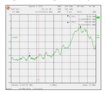
Zigbee Radio transmitting at 2.405 GHz, O-QPSK
