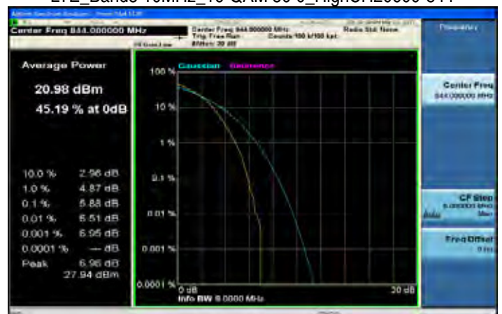
LTE_Band5 10MHz_16-QAM 50 0_HighCH20600-844
