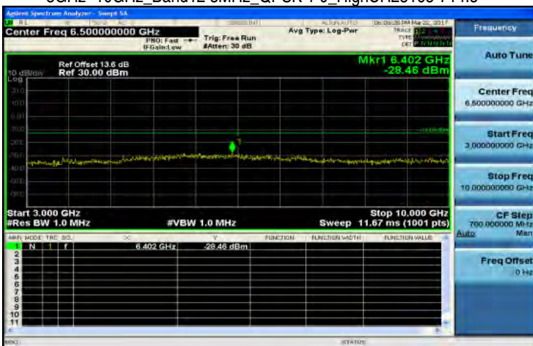
3GHz~10GHz_Band12 3MHz_QPSK 1 0_HighCH23165-714.5
