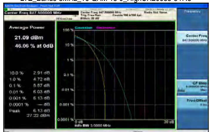
LTE_Band5 3MHz_16-QAM 15 0_HighCH20635-847.5
