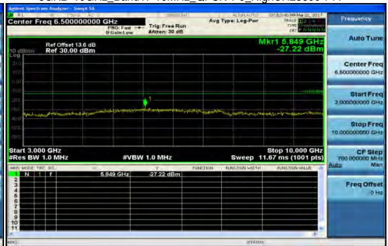
3GHz~10GHz_Band17 10MHz_QPSK 1 0_HighCH23800-711
