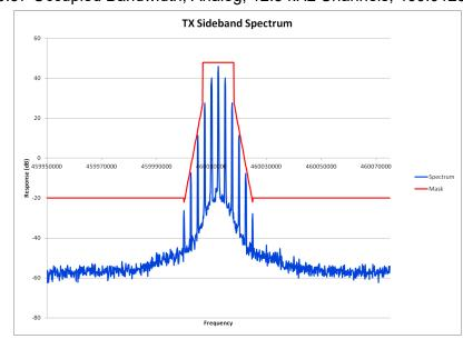
E1-5.37 Occupied Bandwidth, Analog, 12.5 kHz Channels, 460.0125 MHz
