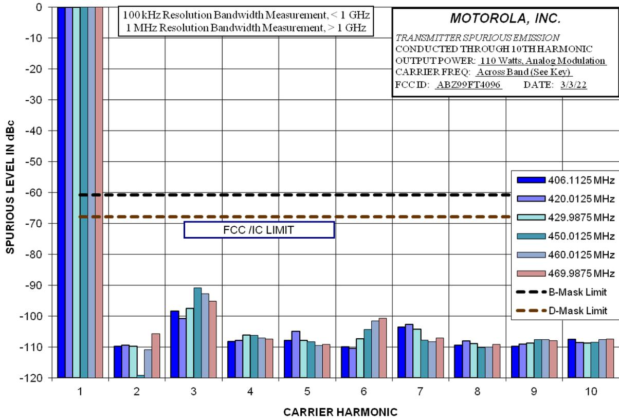
**Report on Test Measurements for FCC ID ABZ99FT4096, HVIN SLR 5700-UHF1 per FCC 47 CFR 90 and IC RSS-119.**
