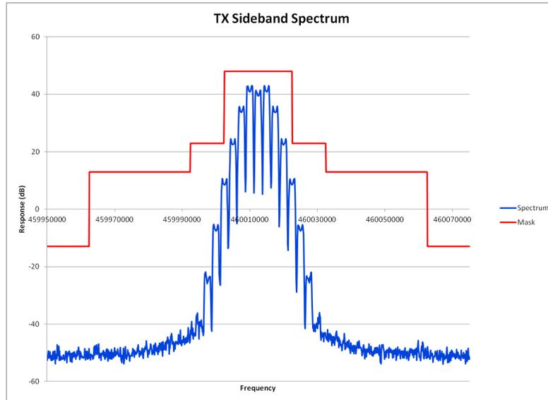
E1-5.22 Occupied Bandwidth, Analog, 25 kHz Channels, 469.9875 MHz
