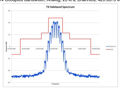
E1-5.15 Occuied Bandwidth, Analog, 25 kHz Channels, 429.9875 MHz DPL
