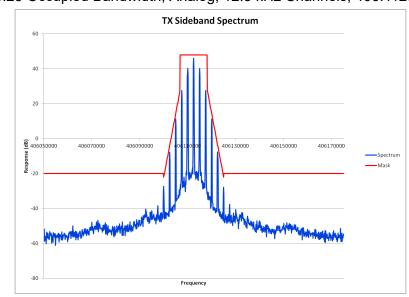
E1-5.25 Occupied Bandwidth, Analog, 12.5 kHz Channels, 406.1125 MHz
