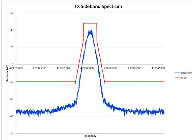
**E1-5.4 Occupied Bandwidth – MOTOTRBO™ Digital Modulation, 450.0125 MHz**
