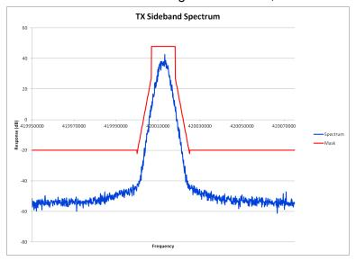
E1-5.3 Occupied Bandwidth – MOTOTRBO<sup>™</sup> Digital Modulation, 429.9875 MHz
