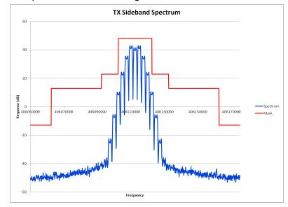
E1-5.9 Occupied Bandwidth, Analog, 25 kHz Channels, 406.1125 MHz DPL
