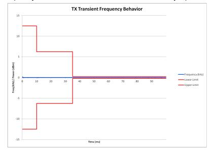
E1-9.17 Frequency Transient Behavior, 12.5 kHz Channel Key-Up, 460.0125 MHz
