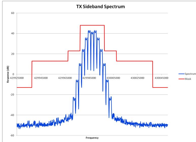
E1-5.16 Occupied Bandwidth, Analog, 25 kHz Channels, 450.0125 MHz
