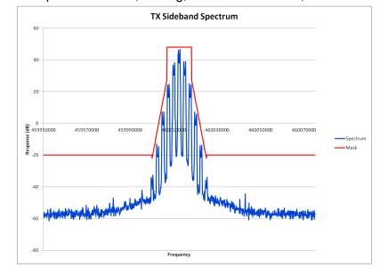
E1-5.39 Occupied Bandwidth, Analog, 12.5 kHz Channels, 460.0125 MHz DPL
