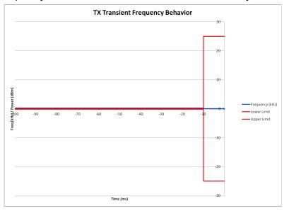
E1-9.7 Frequency Transient Behavior, 25 kHz Channel De-Key, 406.1125 MHz
