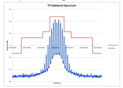
E1-5.19 Occupied Bandwidth, Analog, 25 kHz Channels, 460.0125 MHz
