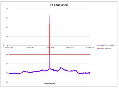
E1-6.6 Conducted Spurious Emission Spectrum, 200 MHz Span, Power 60 Watts, 450.0125 MHz
