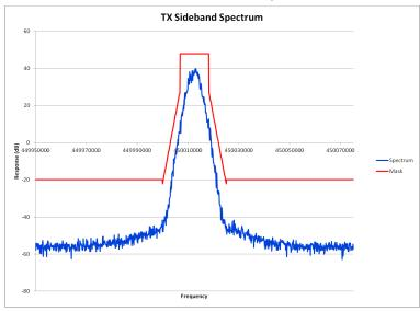
E1-5.5 Occupied Bandwidth – MOTOTRBO<sup>™</sup> Digital Modulation, 460.0125 MHz
