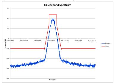
E1-5.1 Occupied Bandwidth – MOTOTRBO<sup>™</sup> Digital Modulation, 406.1125 MHz
