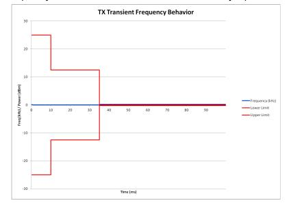
E1-9.5 Frequency Transient Behavior, 25 kHz Channel Key-Up, 460.0125 MHz
