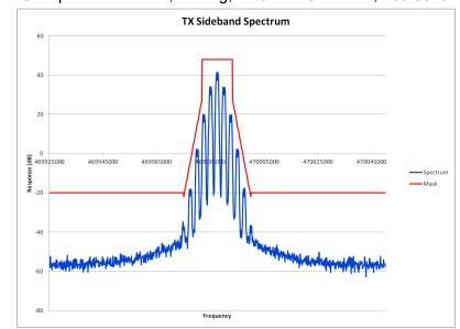
E1-5.41 Occupied Bandwidth, Analog, 12.5 kHz Channels, 469.9875 MHz PL
