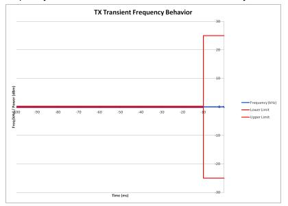
E1-9.9 Frequency Transient Behavior, 25 kHz Channel De-Key, 429.9875 MHz
