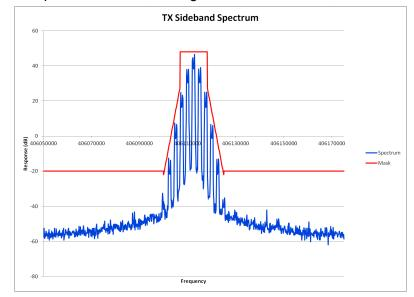
E1-5.27 Occupied Bandwidth, Analog, 12.5 kHz Channels, 406.1125 MHz DPL
