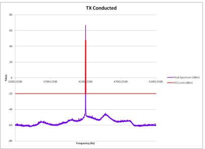
E1-6.5 Conducted Spurious Emission Spectrum, 200 MHz Span, Power 60 Watts, 429.9875 MHz
