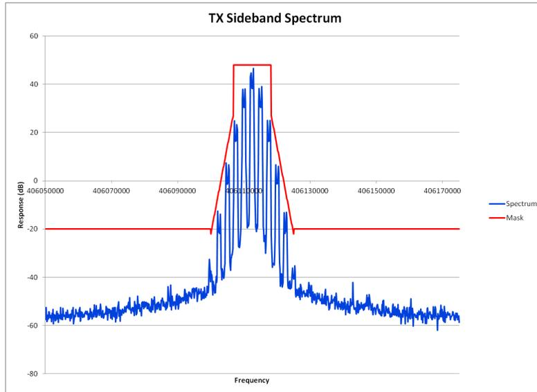
E1-5.28 Occupied Bandwidth, Analog, 12.5 kHz Channels, 420.0125 MHz
