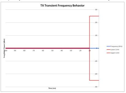
E1-9.11 Frequency Transient Behavior, 25 kHz Channel De-Key, 460.0125 MHz
