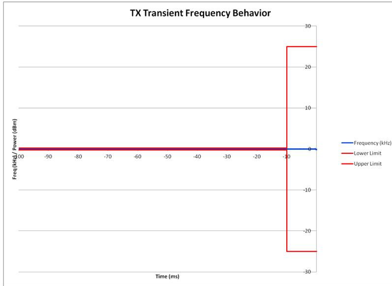
**E1-9.12 Frequency Transient Behavior, 25 kHz Channel De-Key, 469.9875 MHz**
