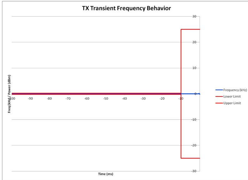
**E1-9.10 Frequency Transient Behavior, 25 kHz Channel De-Key, 450.0125 MHz**
