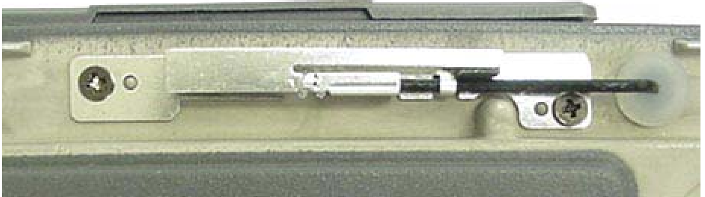
WLAN Antenna 2 (Transmit / Receive)
