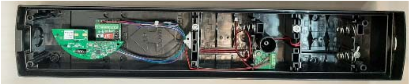
Photograph No.4 PG9350SL Receiver Back Box front view
