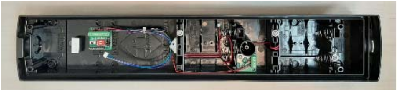
Photograph No.6 PG9350SL Receiver Back Box with RF module removed
