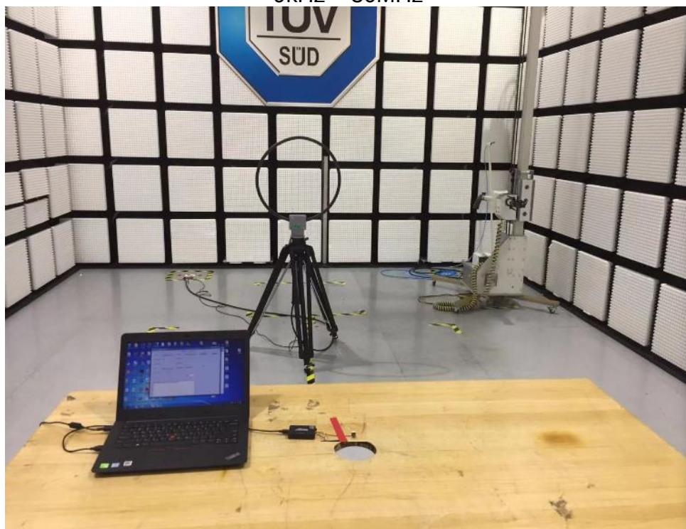
Radiated Emission Setup 9kHz ~ 30MHz
