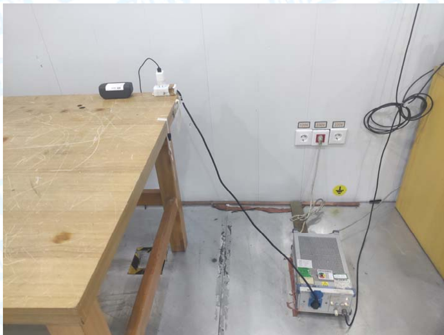
Photo of Setup for Conducted Emission
