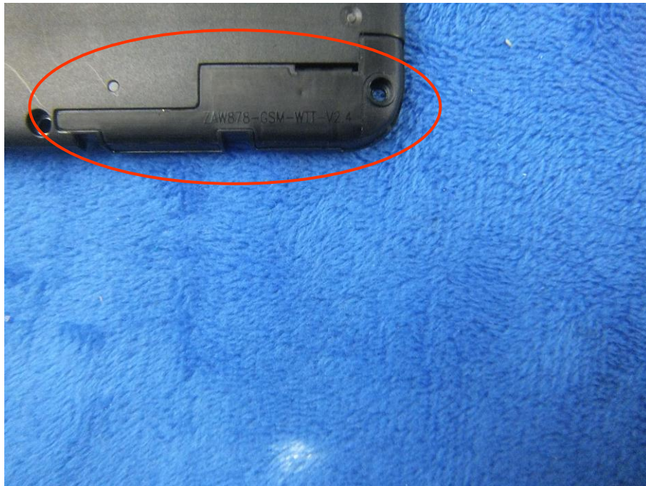
GSM/PCS/UMTS - Antenna View
