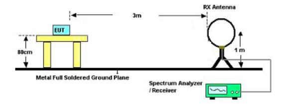
For Radiated Emissions: 30MHz~1GHz
