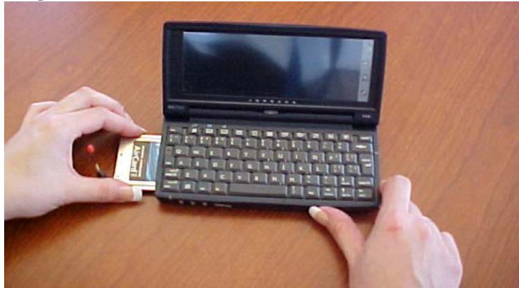
Figure 4-2: Inserting the AirCard into a Handheld PC
