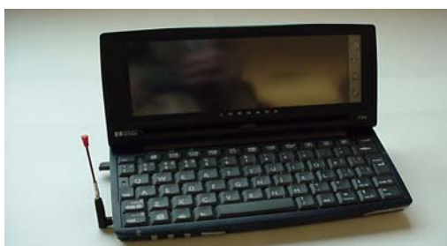
Figure 6-1: Proper positioning of the AirCard antenna
