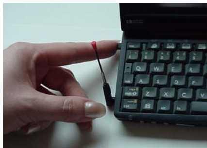
Figure 6-4: Ejecting the AirCard from its slot
