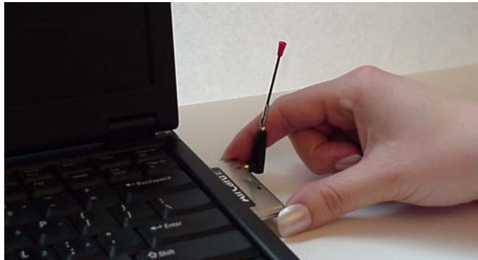
Figure 3-2: Inserting the AirCard
