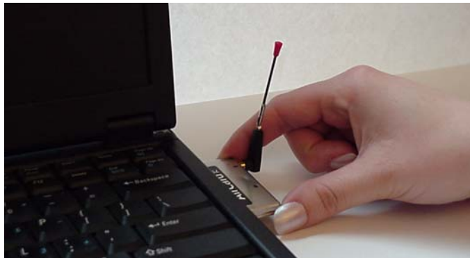
Figure 3-3: Inserting the AirCard
