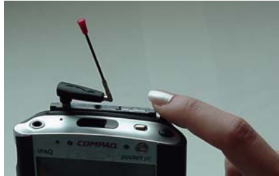
Figure 6-3: Removing the AirCard from its slot (Pocket PC)
