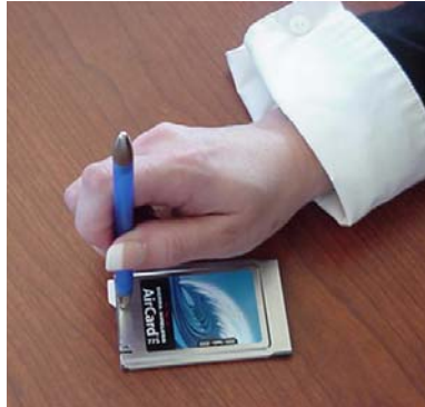
Figure 2-4: Ejecting the SIM card
