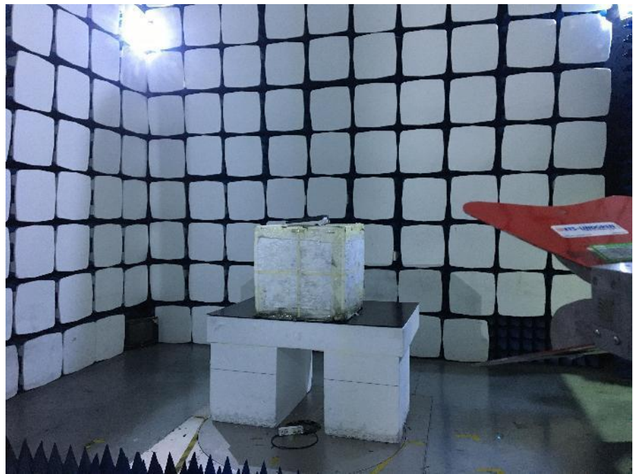
Radiation Emission Test Setup (1GHz to 18GHz)
