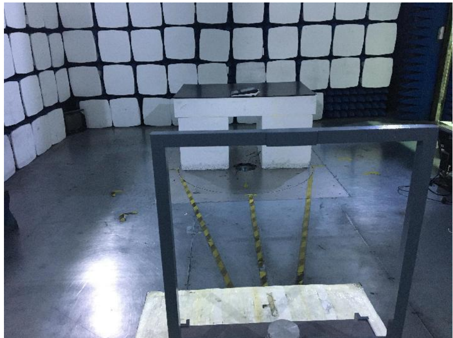
Radiation Emission Test Setup (Below 30MHz)
