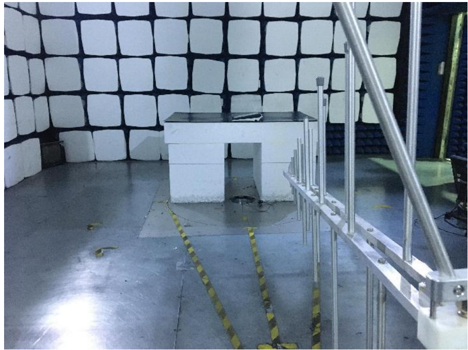
Radiation Emission Test Setup (30MHz to 1GHz)
