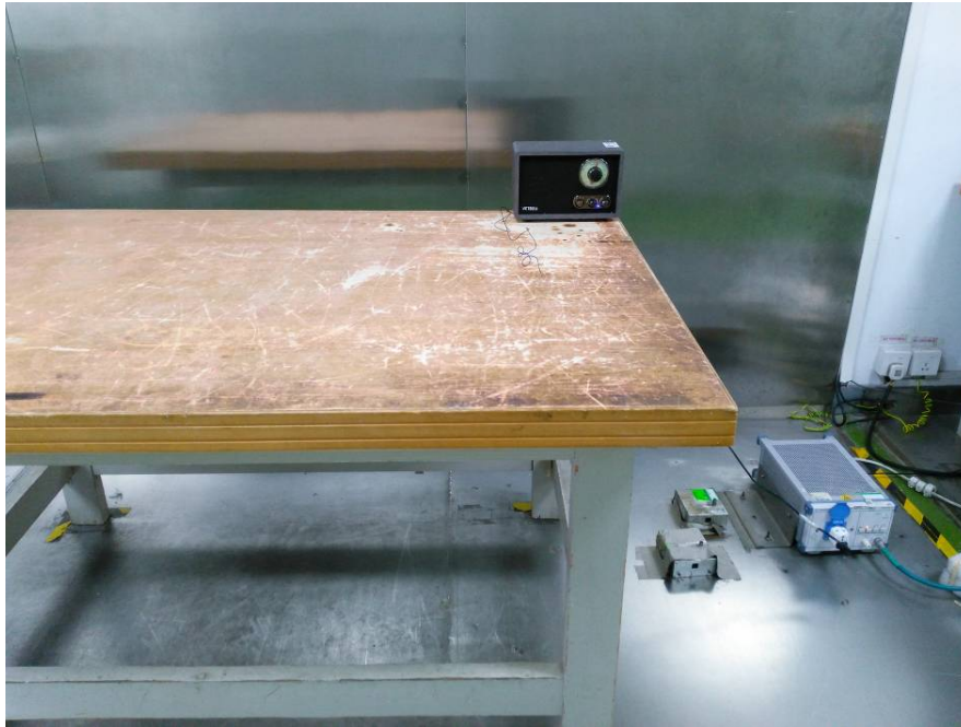
Conducted Emissions - Front View
