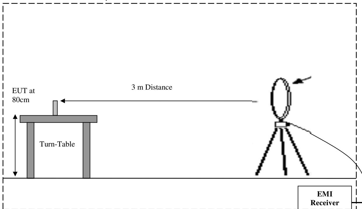
Radiated Emissions Test Setup 30MHz-1GHz Measurements
