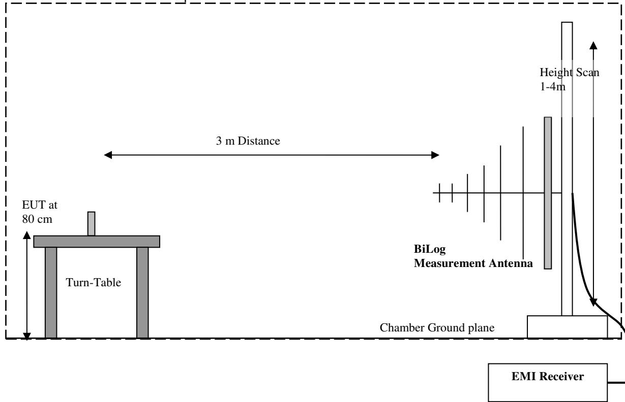
Radiated Emissions Test Setup above 1GHz Measurements
