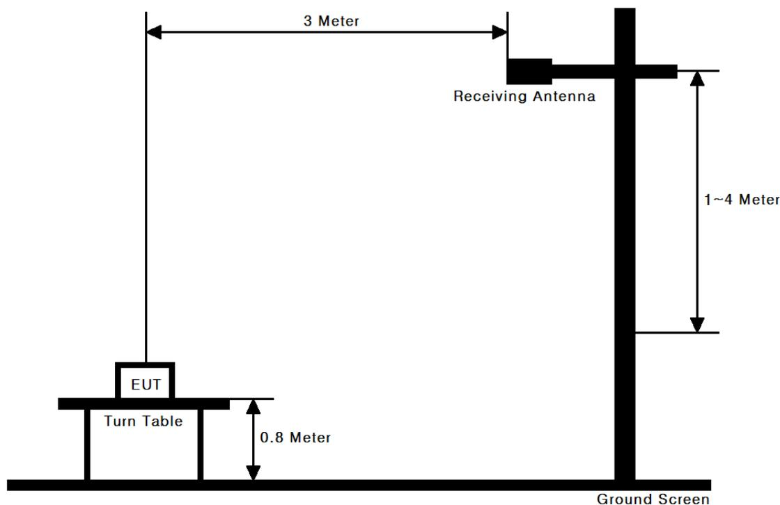
These measurements were performed at 3&10m test site. The equipment under test is placed on a non-conductive turntable 0.8-meters above the ground plane and 3-meters from the receive antenna.
