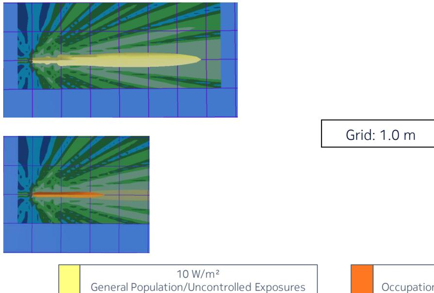
Figure 3 – Power density from AWKUC/D for the actual maximum transmitted power of 4.2 W (corresponding to the actual EIRP threshold of 66.25 dBm) and the beam oriented in azimuth = 0° & elevation = 0° (top view)
