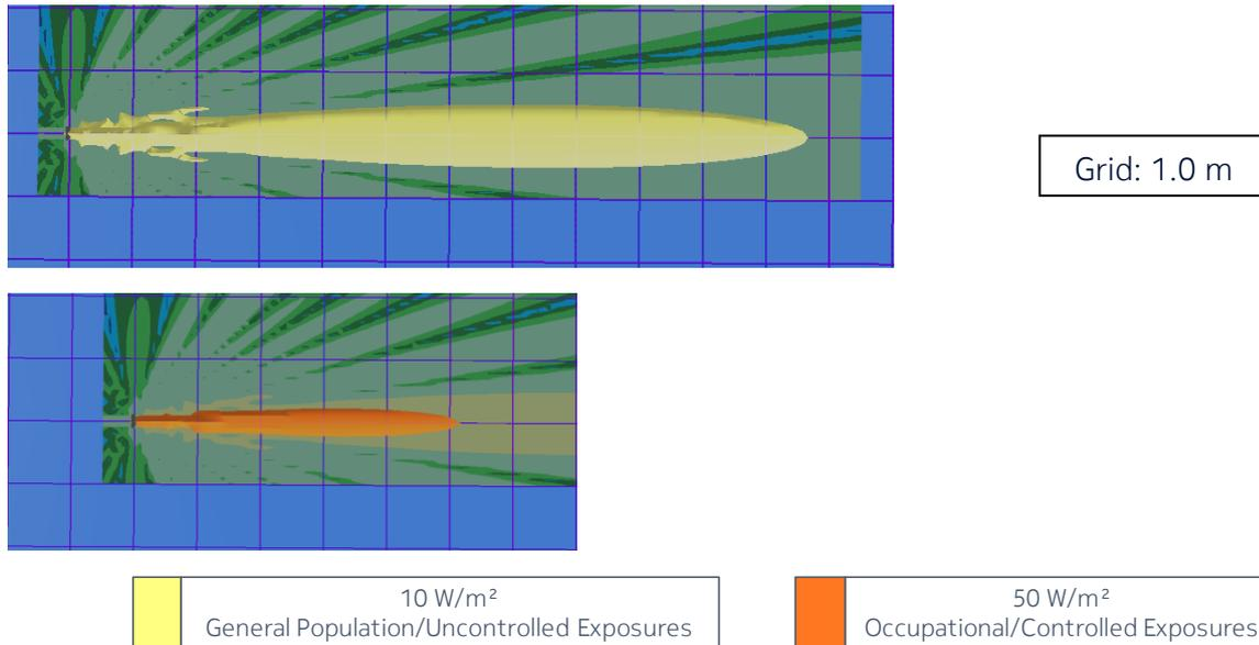
Figure 2 – Power density from AWKUC/D for the time-averaged maximum transmitted power of 16.8 W (corresponding to the time-averaged maximum EIRP of 72.25 dBm) and the beam oriented in azimuth = 0° & elevation = 0° (top view)
