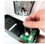
Insert the cable into the connector
