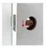
Use self-tapping screws to fix the lock body gusset box to the lock body small hole downward ↓As shown in Figure 1
