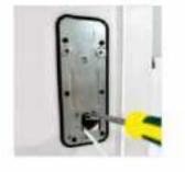
Align the holes of the built-in board and fix them with flat head screws
