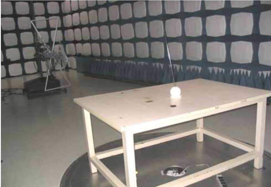
Radiation Emission Test setup
