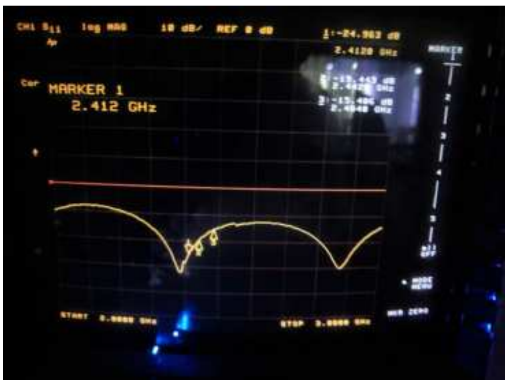
FIG 3 EWN-8822CSS3AH 2.4G Path B
