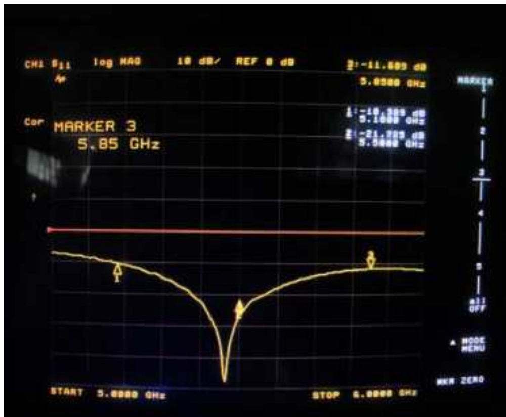
FIG 4 EWN-8822CSS3AH 5G Path A
