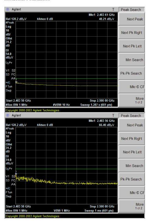
Co-location Radiated Emissions 2462 MHz and 5805 MHz, Ave and Pk Horizontal Polarization
