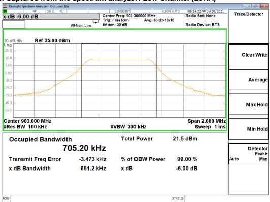
Screen Captures from the spectrum analyzer: MID Channel (LoRA)
