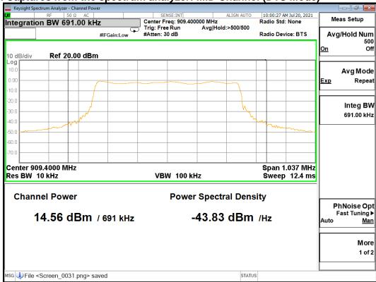
Screen Captures from the spectrum analyzer: High Channel (DTS Mode)
