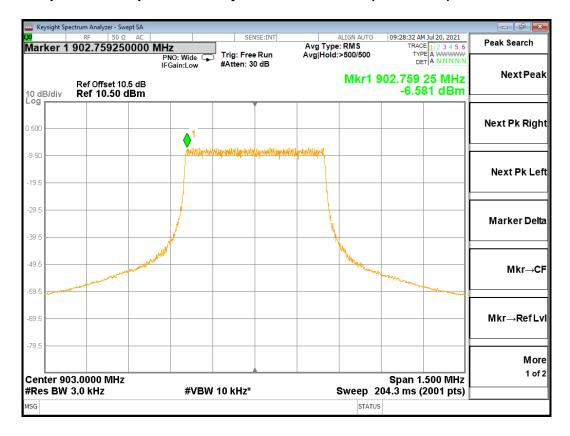
Screen Capture from Spectrum Analyzer: MID Channel (DTS Mode)
