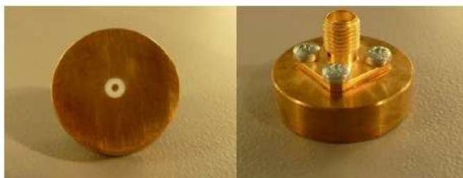
Figure 1 – MVG LIMESAR Dielectric Probe
