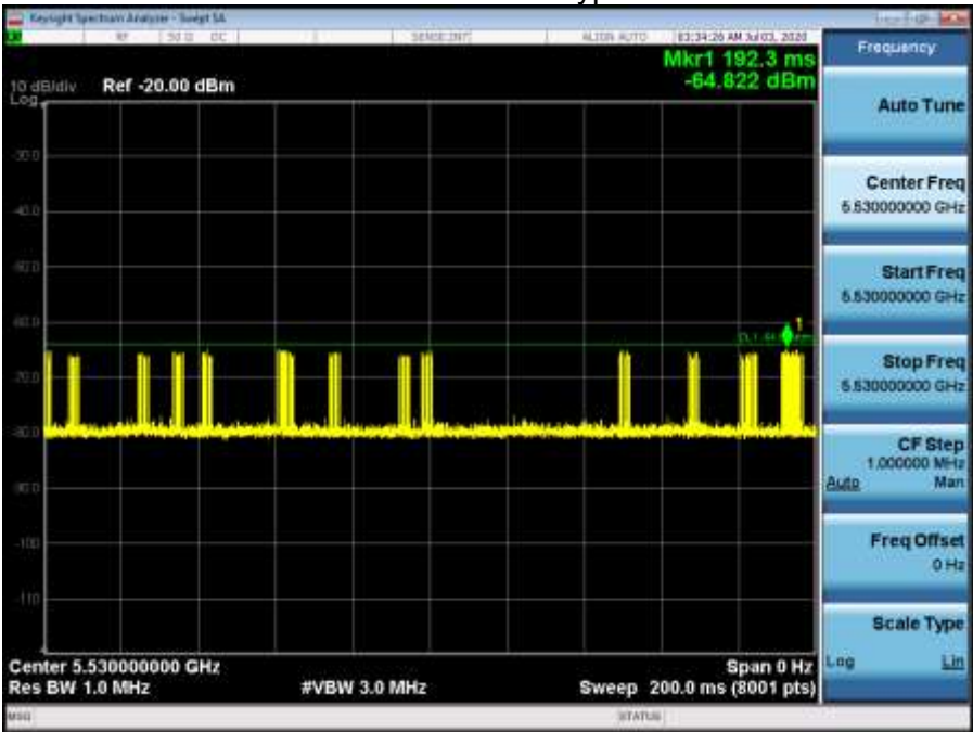
11ac80 CH106 5530MHz Radar Type 6 Calibration Plot
