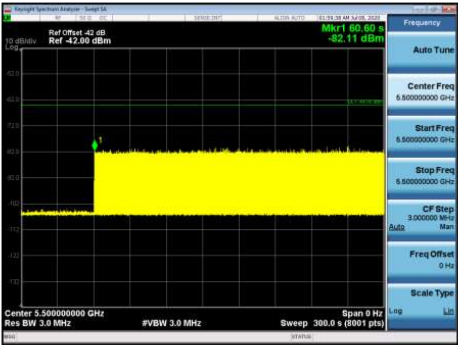
Initial Channel Availability Check Time AP460S6C 11a CH100 5500MHz
