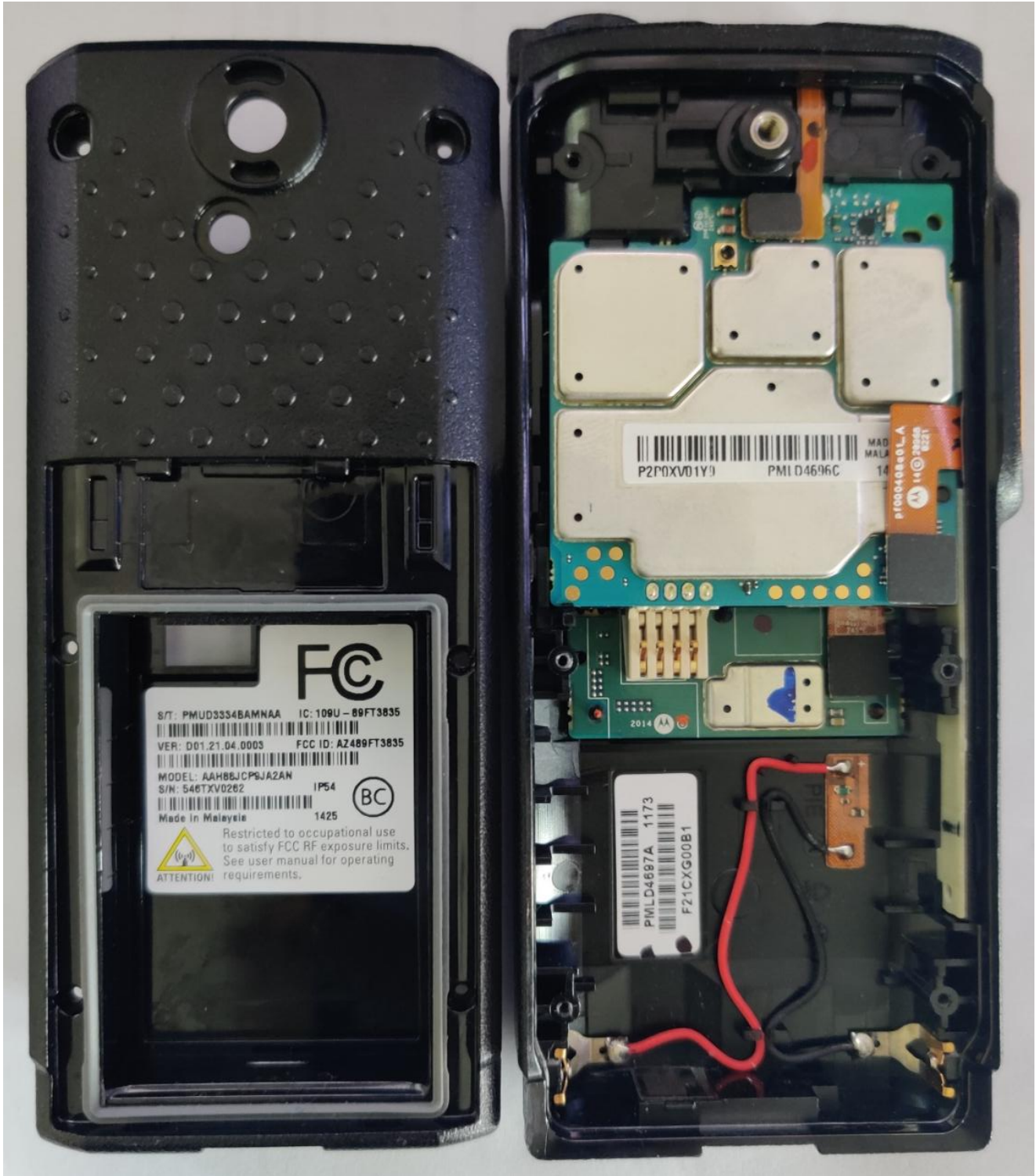
PCB board with chassis and housing for Display Model (Bottom)
