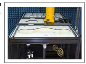
The device holder positions are adjusted to the standard measurement positions in the three sections. A cover is provided to tap the phantom during off-periods to prevent water evaporation and changes in the liquid parameters. On the phantom top, three reference markers are provided to identify the phantom position with respect to the robot.
