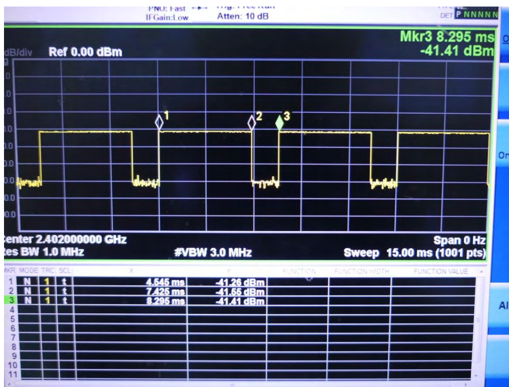
Time-domain plot for Bluetooth transmission signal
