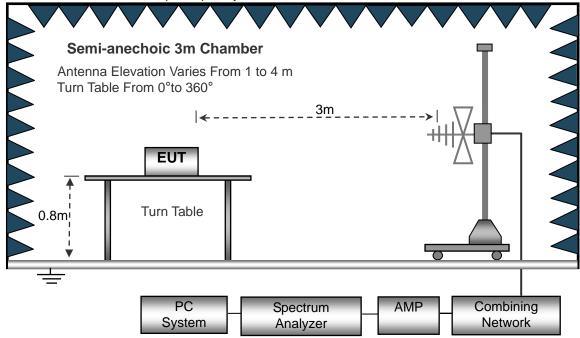
(C) Radiated Emission Test-Up Frequency Above 1GHz
